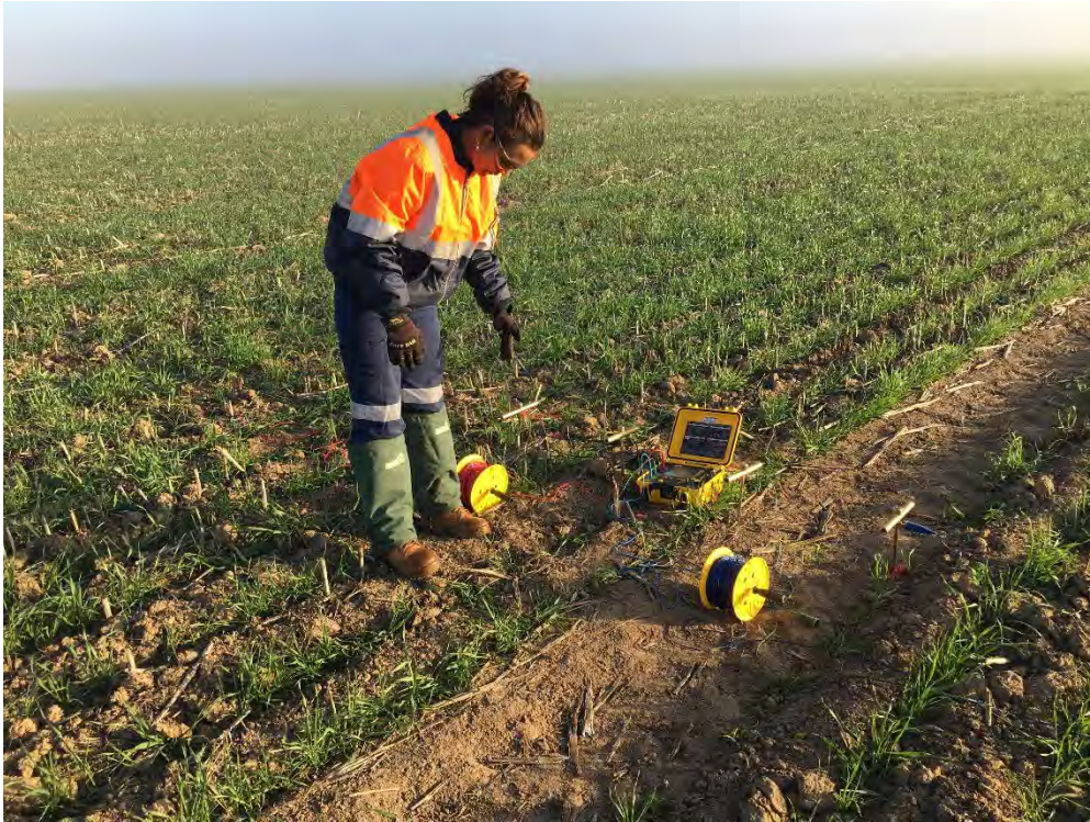
Figure 3: Testing process- AEMC 6472 Ground Tester
