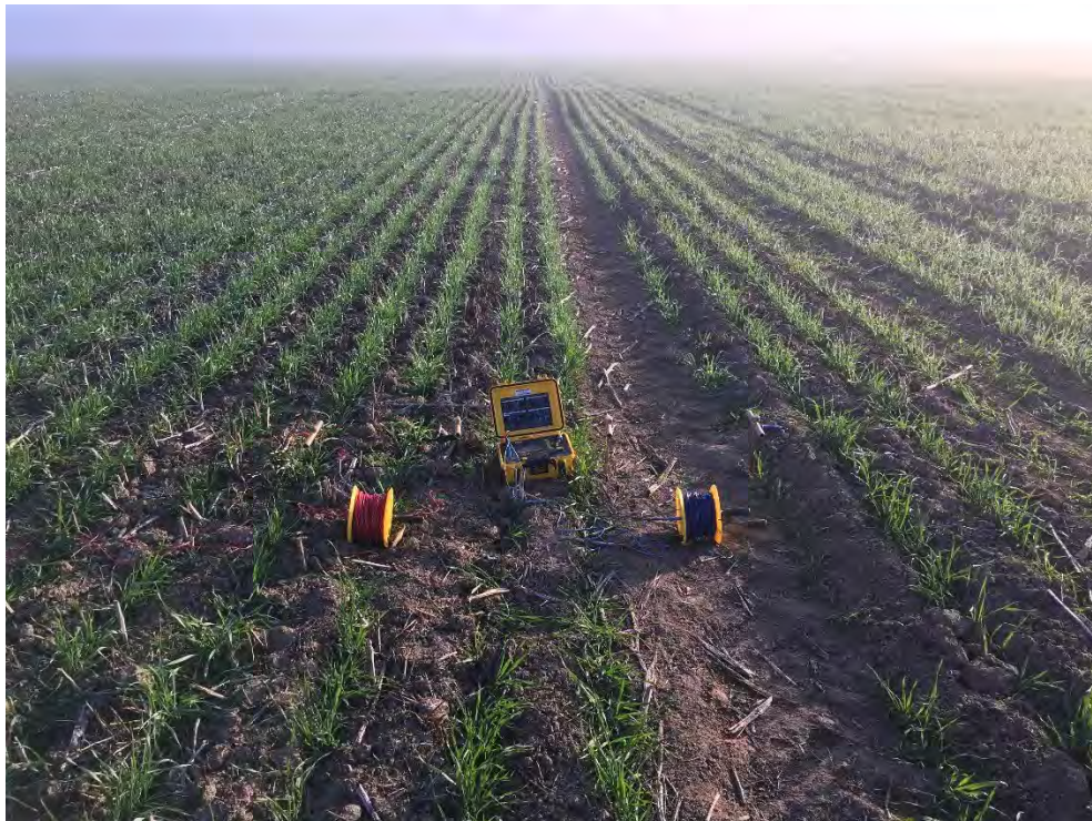
Figure 4: Testing process - indicating probe layout and using AEMC 6472 Ground Tester
